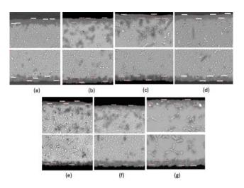
**Figure 9.** Intermetallics and microstructure for: a) SAC105, b) SAC125N, c) SACX Plus 0307, d) SAC305, e) Innolot, f) Maxrel Plus (SAC305 paste), and g) Maxrel Plus (Maxrel<sup>TM</sup> Plus paste). PCB at the bottom.
