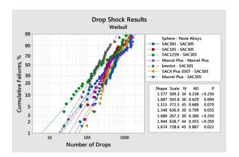
Figure 6. Drop shock performance of sphere-solder paste combinations
