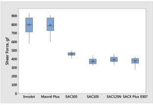
Figure 5. Single ball shear strength
