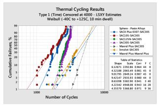
Figure 7. Weibull curves of thermal cycling test results
