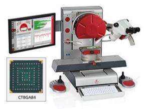
Figure 1. Condor Sigma bond tester. CTBGA84 (inset)
