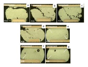
**Figure 8.** Cross-sections after 4,000 thermal cycles. a) SAC105, b) SAC125N, c) SACX Plus 0307, d) SAC305, e) Innolot, f) Maxrel Plus (SAC305 paste), and g) Maxrel Plus (Maxrel Plus paste)
