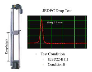
**Figure 3.** Lansmont drop shock testing machine (left) and half-sine shock pulse curve (right)
