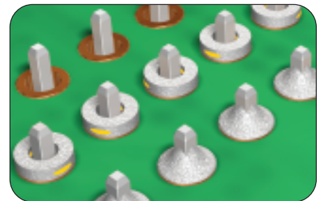
Bare pins, washers in place pre-reflow, post-reflow
