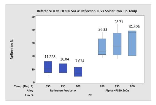
Figure 3 – Reflectivity Results of HF850 vs Reference Cored Wire
